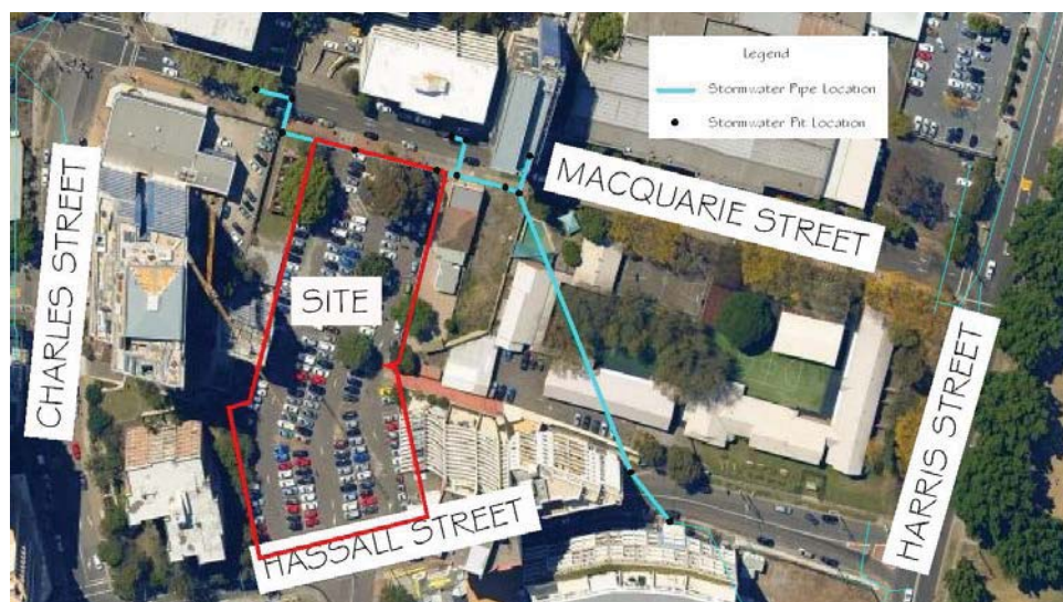
Figure 3.2 – Stormwater Drainage Layout
